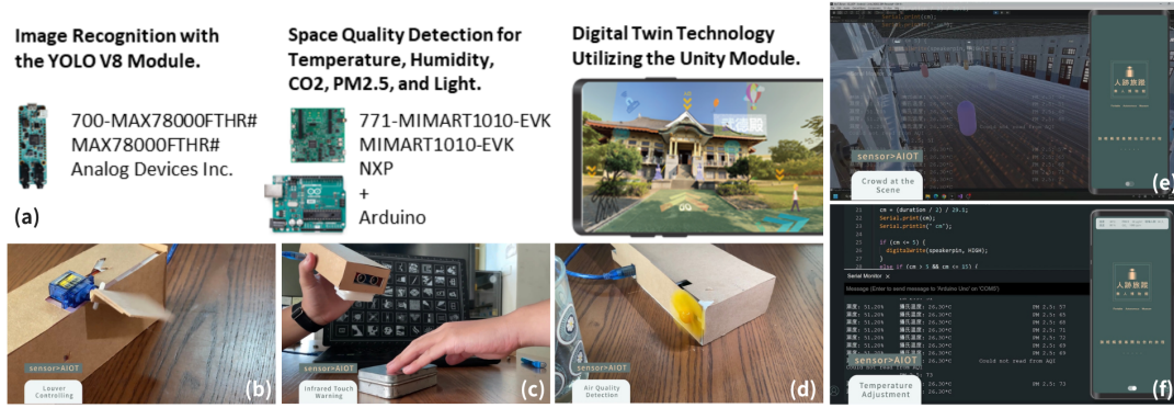
Figure 6: SensorHub: (a) Microcontrollers and Sensors, (b) Louver Controlling, (c) Infrared Touch Warning, (d) Air Quality Detection, (e) # of Crowds, and (f) Temperature Adjustment.
